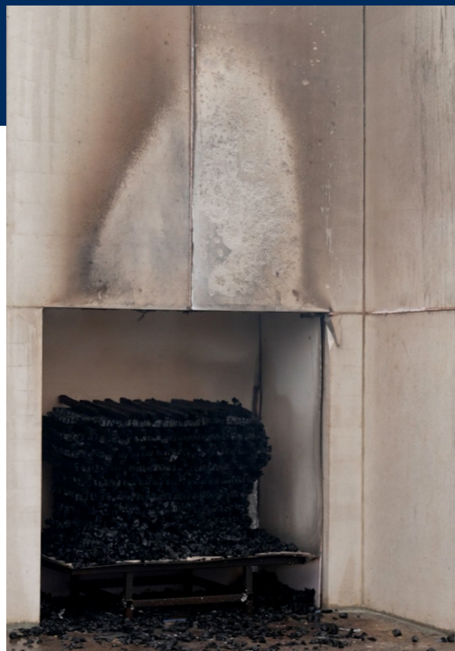
Figure 4. Panels once the fire had been extinguished after 30 minutes
